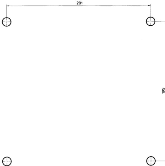
The diameter of the hole depends on the screws used (max. screw diameter 8 mm) and the type of the surface (steel, wood, concrete, sheetrock etc.) and please select accordingly.
