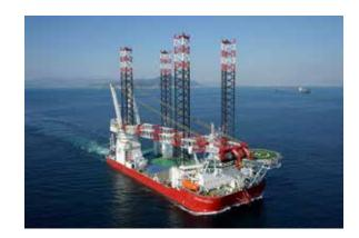
This vessel is based on the Gusto MSC NG14000X design, the ABS-classed Seajacks Scylla, has more than 8,000 metric tons of available variable deck load. Equipped with a 1,540-metric-ton leg-encircling crane and a usable deck space in excess of 5,000 square meters the unit is outfitted with 105-meter legs with the ability to install components in water depths to 65 meters. The rig is capable of meeting the installation
